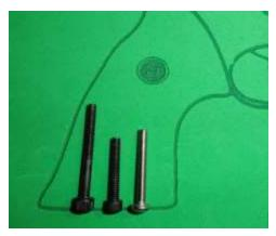
The standard Dan Wesson grip screw size is either 1  $\frac{1}{2}$ " or 1" in length with an 8-32 thread. Since the thread is a common size, easily found at a hardware store, the Dan Wesson owner may discover they have something different than standard, such as a 1  $\frac{1}{4}$ " pan head screw. Any screw that properly fits is just fine.
